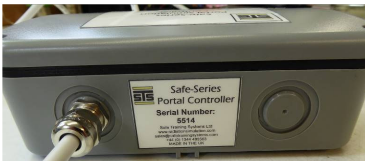
Cable to Portal Detector
